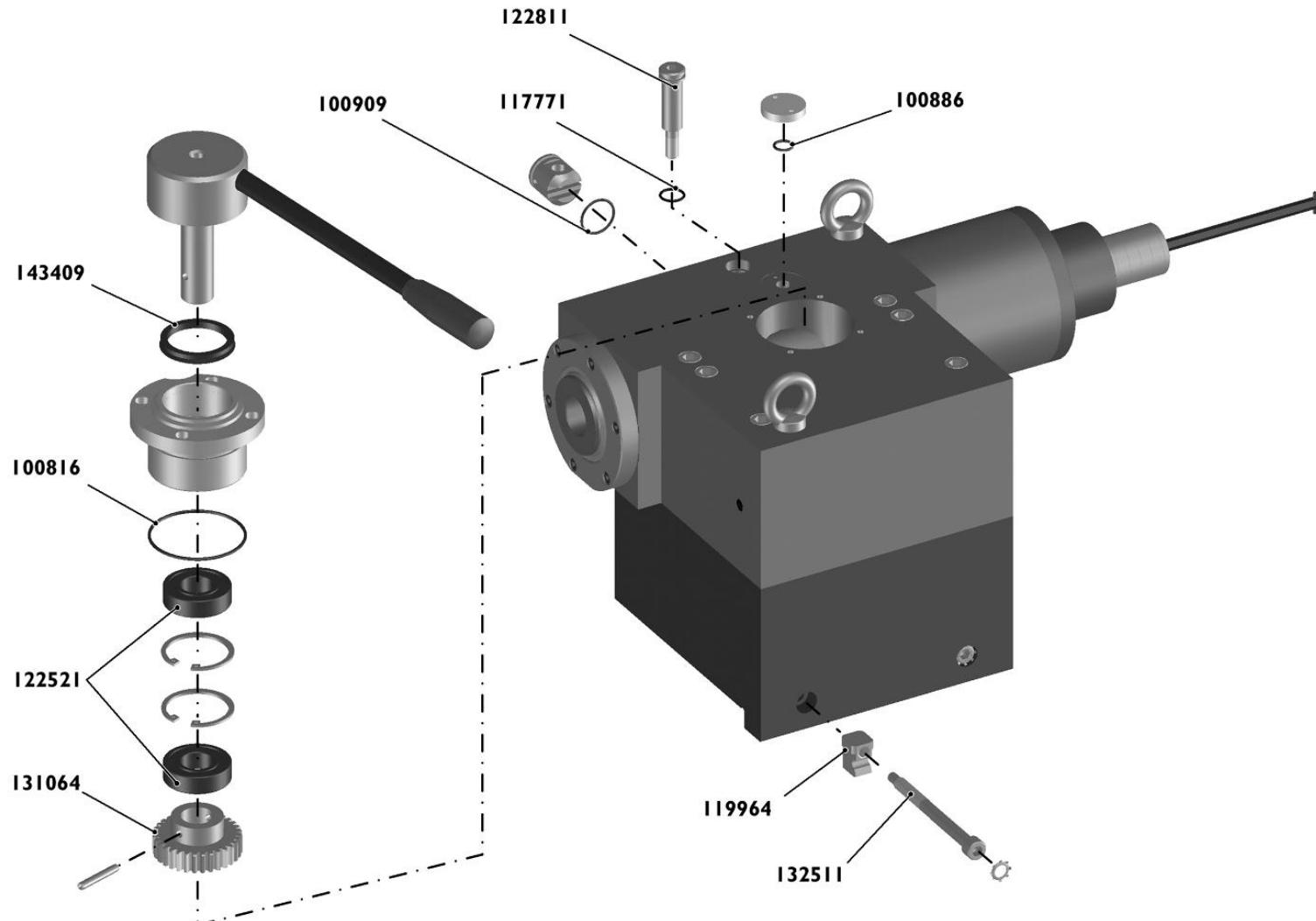
**Reitstock verstärkt mit Hydraulikrückzug    Contre-poupée renforcée, rétraction hydraulique    Reinforced tailstock, hydraulic sleeve retraction**
