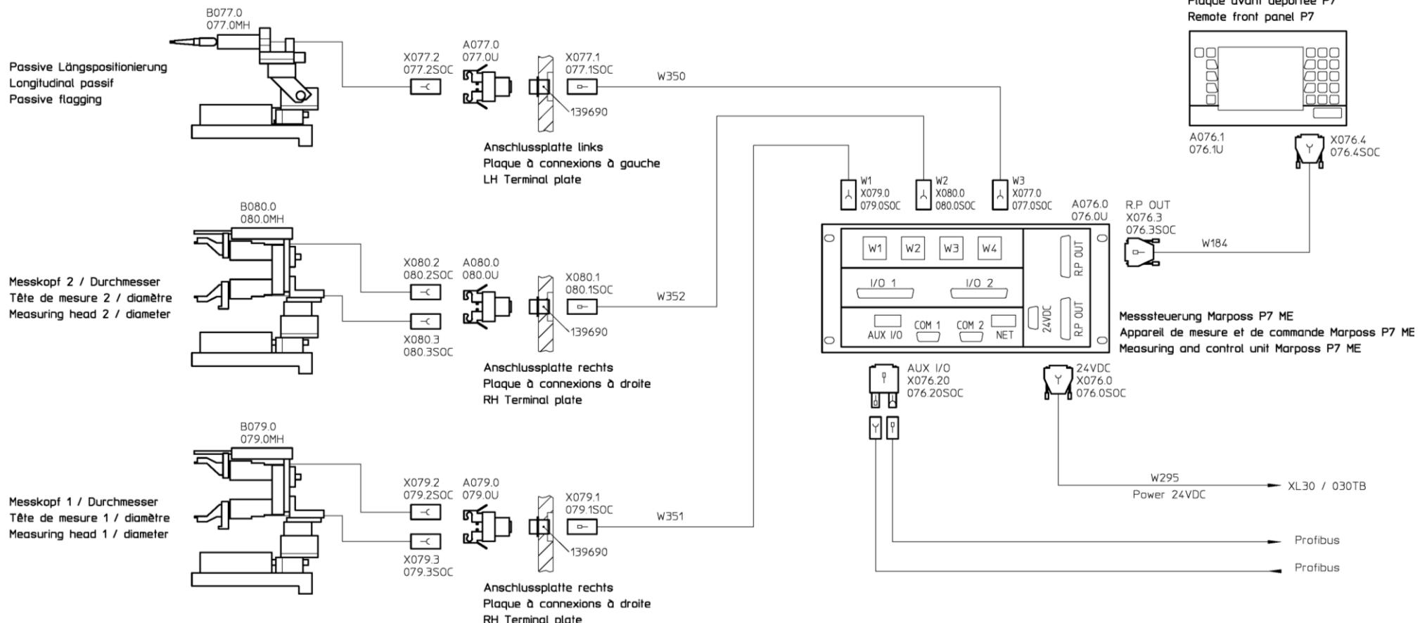
**Hardware Kabel Movomatic ESZ 400    Hardware câble Movomatic ESZ 400    Hardware cable Movomatic ESZ 400**
