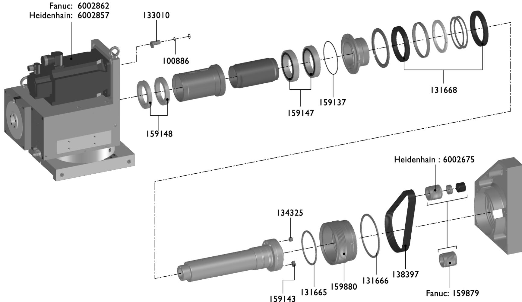
**Werkstückspindelstock verstärkt    Poupée porte-pièce renforcée    Reinforced workhead**
