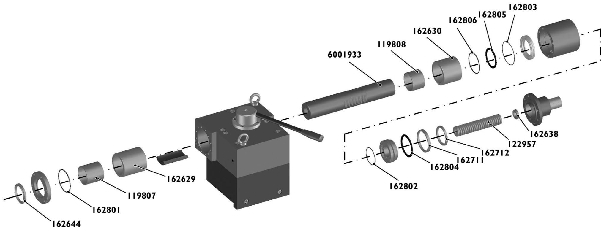
**Reitstock Feinverstellung   Contre-poupée ajustage fin   Tailstock fine adjustment**
