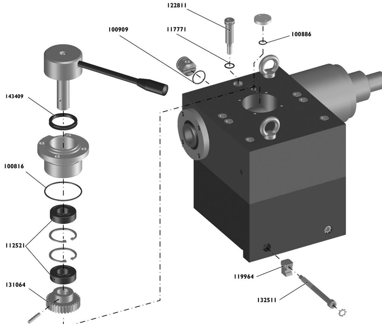
**Reitstock Stand. mit Hydraulikrückzug    Contre-poupée stand. avec rétraction hydraulique    Tailstock stand. version with hydraulic sleeve retraction**
