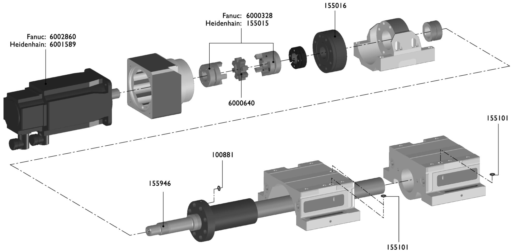
**Schleifschlitten X-Achse   Chariot porte-meule axe X   Grinding slide X-axis**
